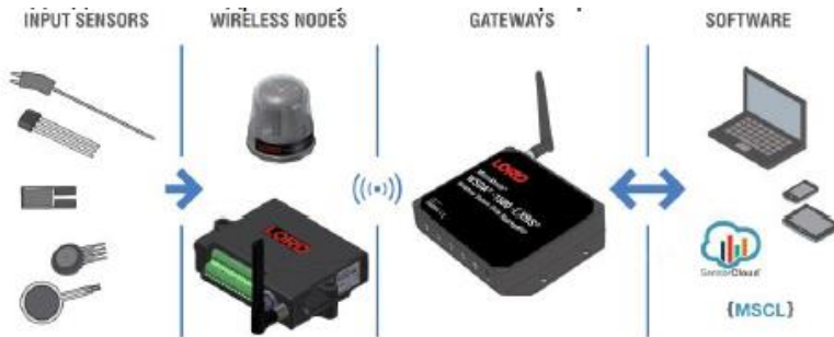
Fig. 1.9 – The general scheme of using LORD sensing systems and IoT technologies
