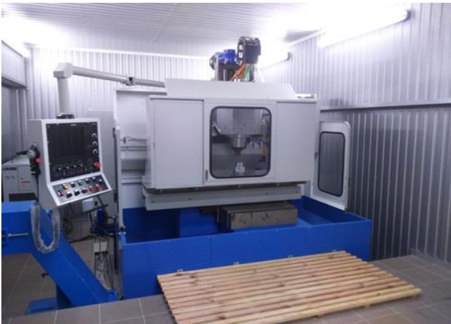
Fig. 2.1 – CNC machine for milling parts of gas turbine engines
