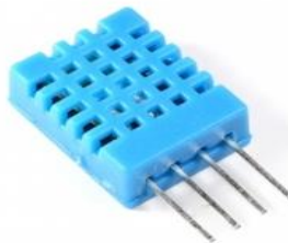
Fig. 5 – Temperature and humidity sensor DHT11
