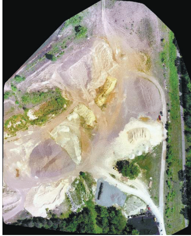
Fig. 1.11 – Overlay of the DSM produced by Pix4D from the images taken by the Phantom drone
