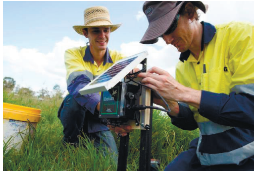
Fig. 3.1 - Libelium sensors and EnviroSuite Agriculture Model being installed at AJ
