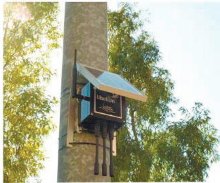
Fig. 2.2 - Waspote Powered by Solar Panel
